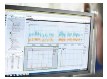
VibGuard IIoT sends measurements to OmniTrend Center software where teams can visualize, evaluate, trend, and store all incoming data. It is compatible with ethernet (TCP/IP), Modbus (TCP/RTU), and MQTT interfaces.
