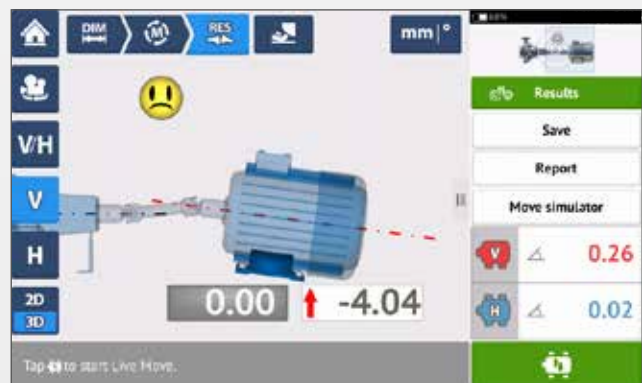
As shafts are rotated, measurement quality is clearly displayed – a green or blue sector indicates good measurement data.
