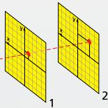
With two position-sensitive detectors and an electronic inclinometer the sensor measures the exact position of the laser beam as the shafts are rotated.
